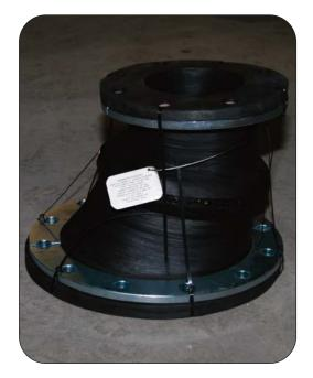
Thorburn's 42HPOX are custom rubber flexible pipes designed to replace rigid piping and absorb axial, lateral and angular movement caused by ground settling of storage tanks. Thorburn's 42HPOX can be manufactured with built in offsets, non parallel flanges with tangents to connect to existing storage tanks where angular and lateral offsets have occurred. Thorburn's 42HPOX can also be designed with multiple filled arches to provide smooth flow and prevent sediment build up in the arches.
