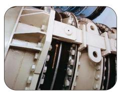
Thorburn's Rubber Hinge Expansion Joints are typically used in sets of two or three, to absorb pipe movement in one or more directions in a single plane piping system. Each individual joint in the system is restricted to pure angular rotation by its hinges.
