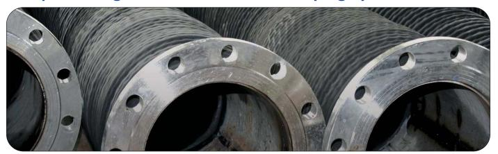
Thorburn 60TMH<sup>™</sup> Flexpipe is a custom designed rubber piping system that replaces metal, rigid or flexible pipe and is used in lines requiring resistance to electrolysis, corrosion, abrasion and water hammering. 60TMH<sup>™</sup> Flexpipe is specifically engineered for piping systems that require isolation and absorption of severe noise, vibration, misalignment, lateral deflection and flexing caused by thermal and mechanical movement.
