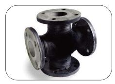
Thorburn's 60TMH<sup>TM</sup> special handcrafted rubber fittings are strong, rugged and flexible. They will reduce noise and vibration from pumps, compressors and other equipment and allow for misalignment where abrasion or corrosion will damage normal piping. Available with tangents and custom offset to absorb extreme angular or lateral deflection in tight spaces.
